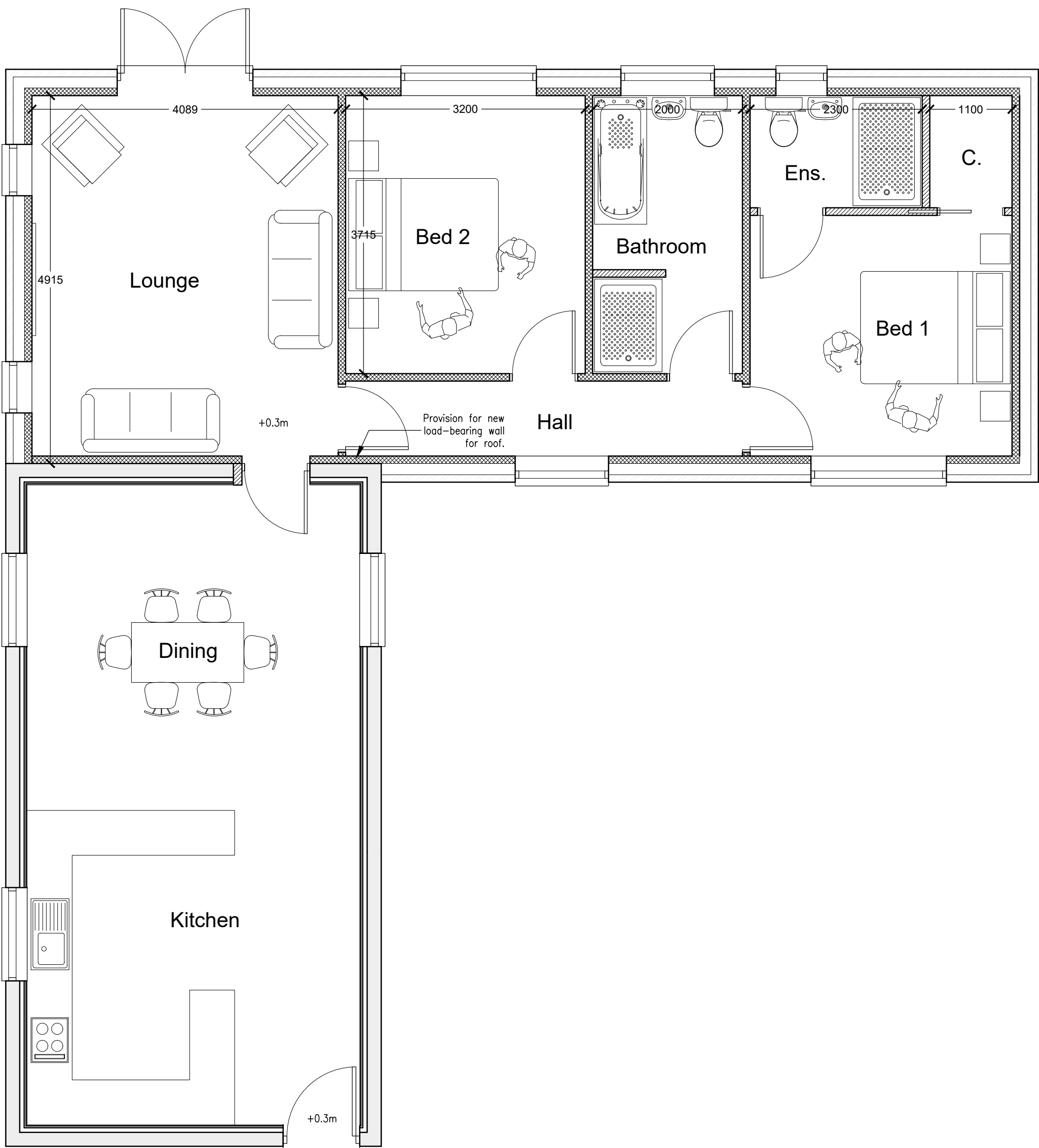
PROPOSED GROUND PLAN 1:50
